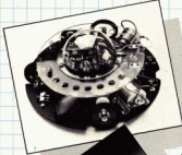
Line Tracer II £17.99 Draw a line and the ultra-red sensor picks it up and sends this 5 wheeled, twin motored robot along the course you plot.
